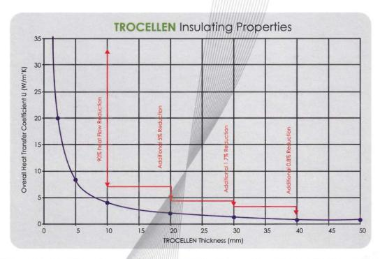
One of the determining factors governing the indoor temperature of a building is the rate of heat flow through the roof structure. Trocellen reduces this heat flow dramatically, even when using low thickness material (10mm Trocellen will block 90% of heat flow).
